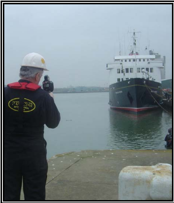
Compact Hand Held Laser Gun, in operation. Sighting Scope with in-scope red dot enables easy aiming. Measurements are displayed on a large LCD display.
