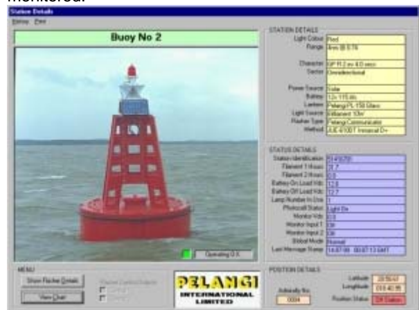
Level 5: Actual site photographs confirm the station being monitored within a standard layout alongside the station's equipment and the active parameters being monitored.
