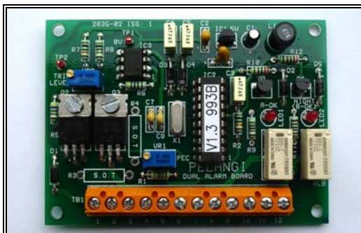
PA2835 Mk 2 Board with second (light status) Relay
