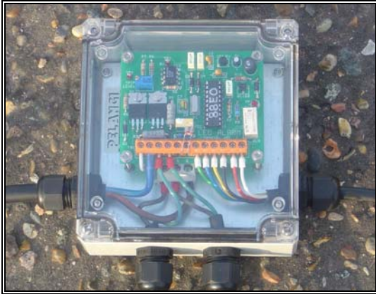
PA2835 Mk 1, and weatherproof junction box
