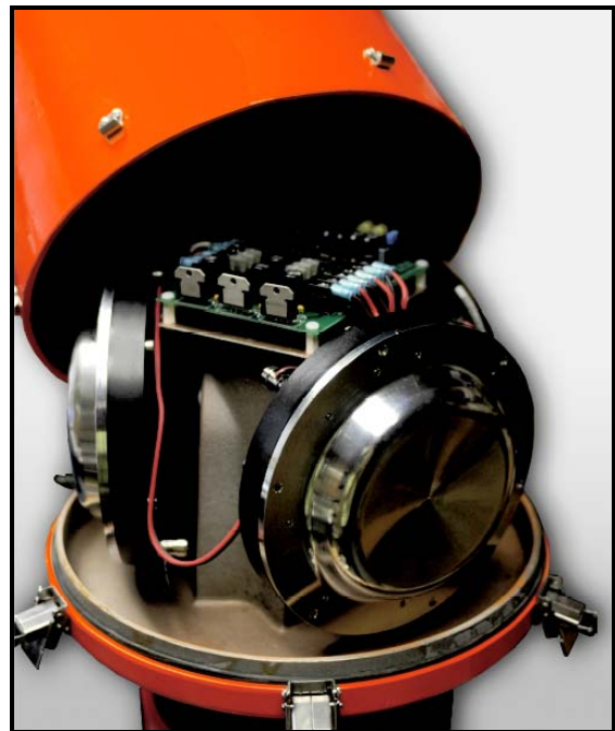
FW3 components including 3 separate drivers for more economical power consumption.
