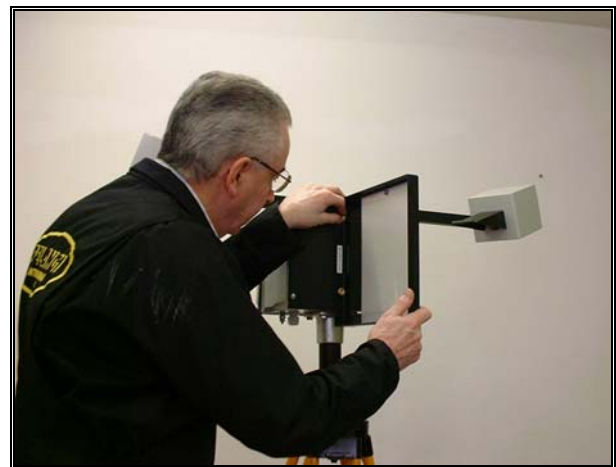
Fitting of scatter plate during calibration procedure
