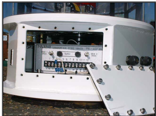
PRL400 Showing one of two access panels, and Easyflash inside the assembly
