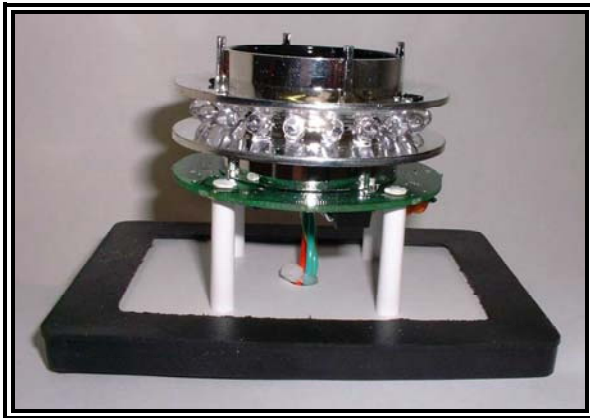
15 L.E.D. Flasher assembly with adjustable flash character
