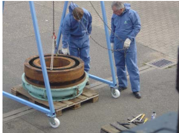
Inner bath being checked for Mercury vapour contamination prior to treatment.
