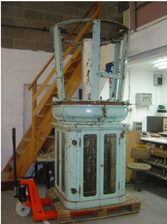
Clockwork, bath and array support at Pelangi works before start of refurbishment and conversion .
