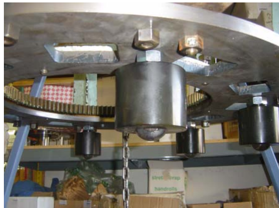
Pre-assembly check of bearings prior to painting .
