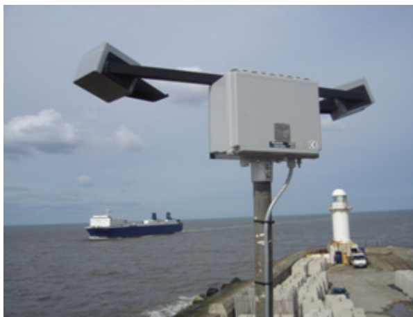
FD7100 Fog detector at South Gare Old Coast Guard Station
