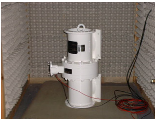
ELG300-2 2 mile 300 hertz 1Kwatt fog horn undergoing test in sound chamber after refurbishment at Pelangi.
