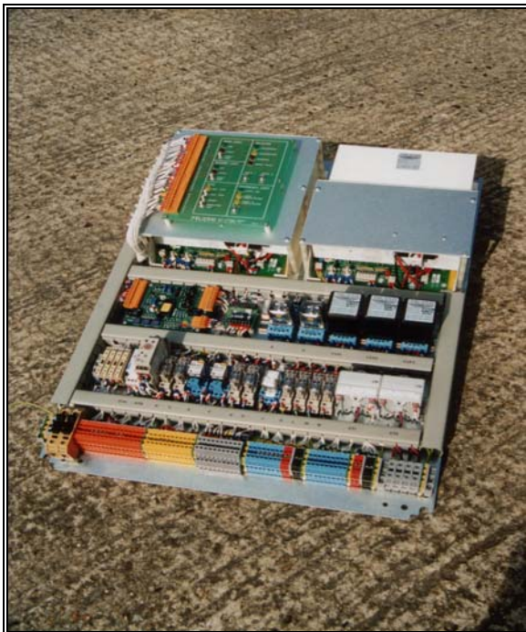
12 volt PRL400 control board with built in dual ballast, LED indicator boards and twin PE cell.
